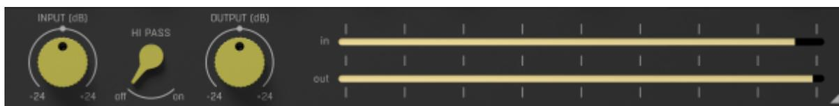
**Input** - controls the input gain in the range of +/-24dB.
